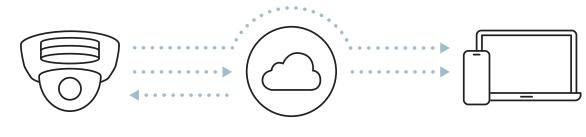
**No NVR or DVRs** Industrial-grade onboard storage saves up to 365 days of continuous video<sup>1</sup> **Easy to scale** Bandwidth friendly and supports thousands of cameras across unlimited locations
